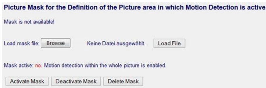
The creation of a mask works simple and quick and can be done by using the Windows Paint Program.
