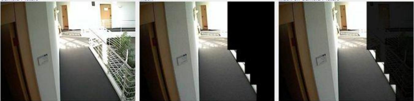
Motion detection is only enabled for the white area of the mask. The complete picture is recorded!
