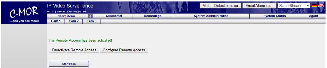
If the data was entered correctly, the remote access is now active and the function can be tested by calling the address <http://remote.c-mor.com:10001>. The password prompt from your C-MOR will appear.
