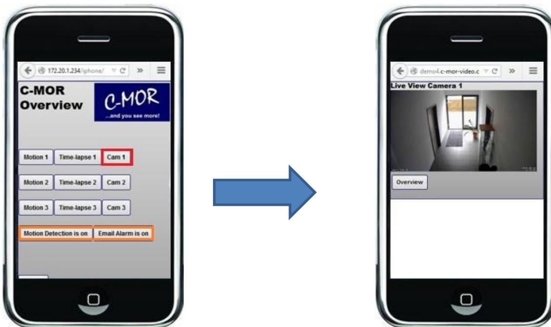
By clicking on the link “Motion <cam no.>” the page with all motion recordings for the selected camera will be opened. By clicking “Time-lapse” the page for all time-lapse recordings of the selected camera will be opened.
