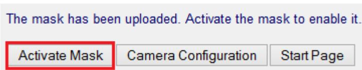
The mask is now activated! Click on "Camera Configuration" to assure the mask is active and is defined for the right motion area:
